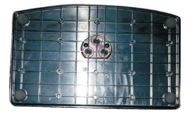
2.To remove the stand, remove the 2 screws in the area and the stand will come off.
